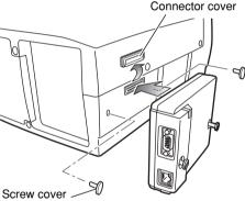
**3** Tighten two screws by using a coin etc.
